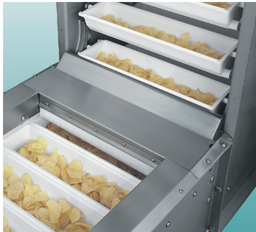
Overlapping buckets prevent product loss during loading.
